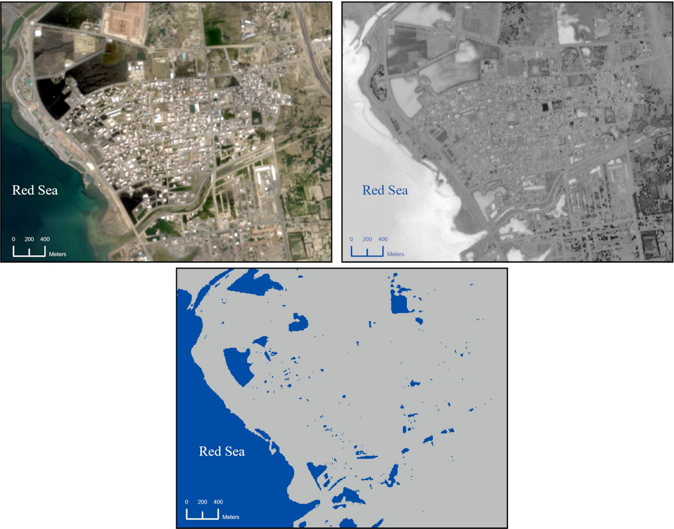
Figure 5. Sentinel-2 true-color image post-flood (top-left); raw hybrid maximum fusion map of ENDWI and AWEIsh (top-right, grayscale normalized); and Otsu-thresholded binary flood map from the hybrid approach (bottom, blue = flooded) for the Al-Lith urban flash flood event. The hybrid method significantly reduces false alarms in built-up areas compared to individual indices.
